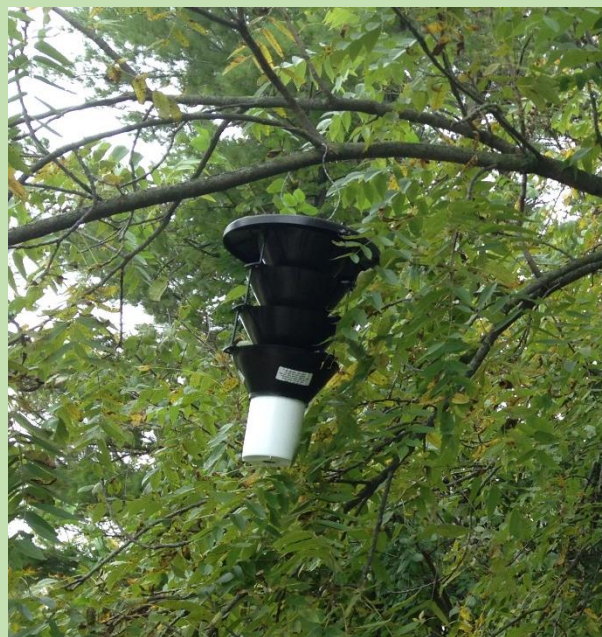
A Lindgren funnel trap, used to monitor for WTB.
